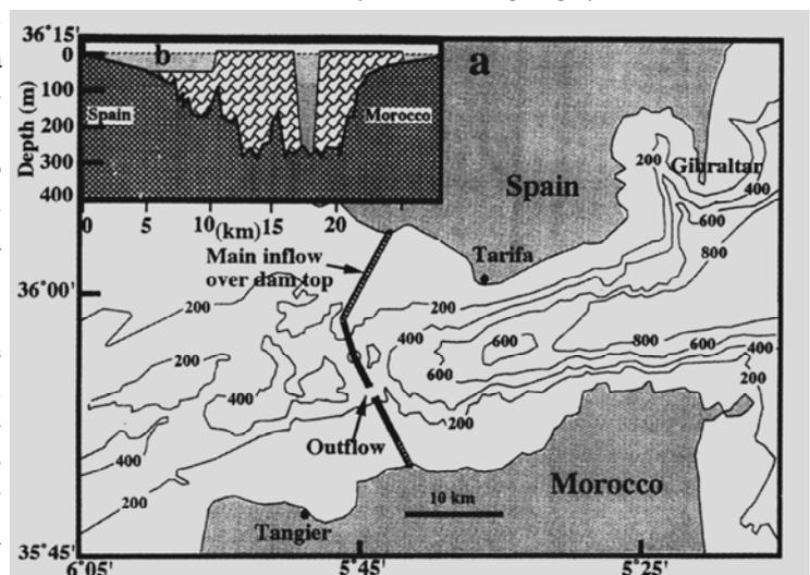
Fig 7 Gibraltar dam with a) Map showing inflow openings and the outflow gate at Camarinal sill b) Transect of the dam (after Johnson 1997)
